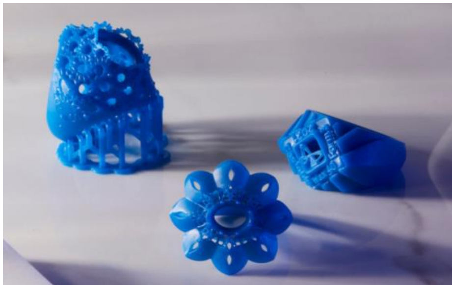
Fig. 3. Items made out of wax-like resin for metal casting [2]
