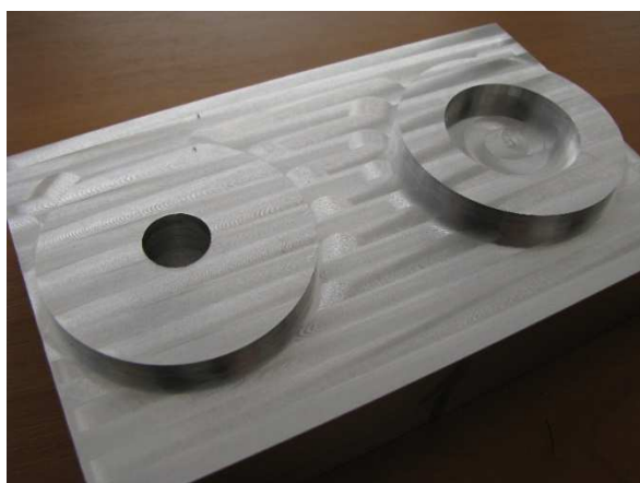
Fig. 2. Example of machined detail on vertical milling center
